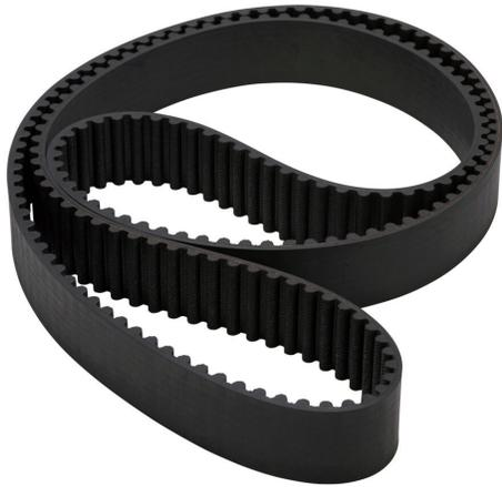
SureMotion timing belt, 8mm 8M pitch, 30mm wide, 189 tooth, 1512mm pitch length (circumference), neoprene, fiberglass reinforced.
