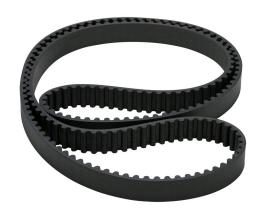
SureMotion timing belt, 8mm 8M pitch, 20mm wide, 189 tooth, 1512mm pitch length (circumference), neoprene, fiberglass reinforced.
