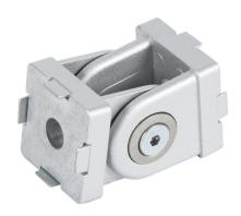
FATH pivot joint, silver, 178-degree adjustable, 2 holes, die-cast zinc, slot size 8. For use with all 30mm and 60mm profile T-slotted rails. Manufacturer part number: 093G30AN08.
