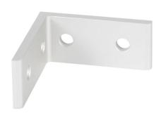
FATH tall inside corner bracket, silver, 90-degree, 4 holes, anodized aluminum, slot size 8. For use with all 30mm and 60mm profile T-slotted rails. Manufacturer part number: 093WD3060.
