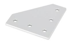
FATH flat plate, silver, 90-degree, 5 holes, anodized aluminum, slot size 8. For use with all 30mm and 60mm profile T-slotted rails. Manufacturer part number: 093VL9090.
