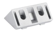
FATH angle connector, silver, 45-degree, 30 x 60mm, die-cast aluminum, slot size 8. For use with all 30mm and 60mm profile T-slotted rails. Manufacturer part number: 093WS60145N08.
