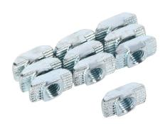
FATH hammer nut, silver, M6-1.0, zinc plated steel, slot size 8. Package of 10. For use with all 30mm and 60mm profile T-slotted rails. Manufacturer part number: 096H08615.
