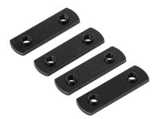
FATH double economy T-nut, black, M6-1.0, zinc plated steel, slot size 8. Package of 4. For use with all 30mm and 60mm profile T-slotted rails. Manufacturer part number: 096E30M6S02R01.
