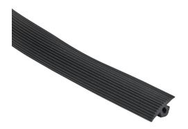
FATH cover profile, black, 6ft, nitrile rubber, slot size 8. For use with all 1.5in, 3in, 40mm and 80mm profile T-slotted rails. Manufacturer part number: 092057.1829.
