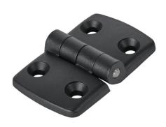
FATH non-detachable combination hinge, black, fiberglass reinforced plastic, slot size 8. For use with all 1.5in, 3in, 40mm and 80mm profile T-slotted rails. Manufacturer part number: 095K4040F08.
