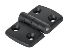
FATH non-detachable combination hinge, black, fiberglass reinforced plastic, slot size 8. For use with all 1.5in, 3in, 40mm and 80mm profile T-slotted rails. Manufacturer part number: 095K4040F08.
