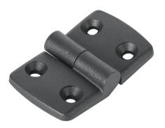
FATH left-hand detachable combination hinge, black, fiberglass reinforced plastic, slot size 8. For use with all 1.5in, 3in, 40mm and 80mm profile T-slotted rails. Manufacturer part number: 095K4040L08.
