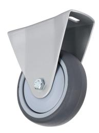
FATH fixed caster, silver/gray, thermoplastic polyurethane/nylon/steel. For use with all 1.5in, 3in, 40mm, 45mm, 80mm and 90mm profile T-slotted rails. Mounting plate included. Manufacturer part number: 098F100U4045N.
