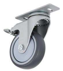
FATH swivel caster, silver/gray, thermoplastic polyurethane/nylon/ steel. For use with all 1.5in, 3in, 40mm, 45mm, 80mm and 90mm profile T-slotted rails. Double brake and mounting plate included. Manufacturer part number: 098S100UD4045N.
