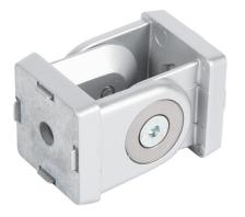
FATH pivot joint, silver, 178-degree adjustable, 2 holes, die-cast zinc, slot size 8. For use with all 1.5in and 3in profile T-slotted rails. Manufacturer part number: 093G38AN08.
