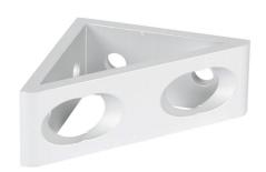
FATH tall gusseted inside corner bracket, silver, 90-degree, 4 holes, anodized aluminum, slot size 8. For use with all 1.5in and 3in profile T-slotted rails. Manufacturer part number: 093W8383N08.
