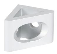
FATH gusseted inside corner bracket, silver, 90-degree, 2 holes, anodized aluminum, slot size 8. For use with all 1.5in and 3in profile T-slotted rails. Manufacturer part number: 093W8384N08.
