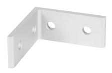
FATH tall inside corner bracket, silver, 90-degree, 4 holes, anodized aluminum, slot size 8. For use with all 1.5in and 3in profile T-slotted rails. Manufacturer part number: 093WD3876.
