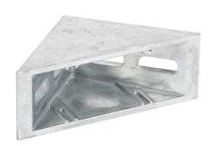
FATH angle bracket, silver, 90-degree, 4 holes, die-cast zinc, slot size 8. For use with all 1.5in, 3in, 40mm, and 80mm profile T-slotted rails. Manufacturer part number: 093W802N08R.
