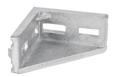
FATH angle bracket, silver, 90-degree, 4 holes, die-cast aluminum, slot size 8. For use with all 1.5in, 3in, 40mm, and 80mm profile T-slotted rails. Manufacturer part number: 093W403N08.
