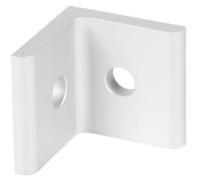
FATH inside corner bracket, silver, 90-degree, 2 holes, anodized aluminum, slot size 8. Package of 10. For use with all 1.5in and 3in profile T-slotted rails. Manufacturer part number: 093WD38.
