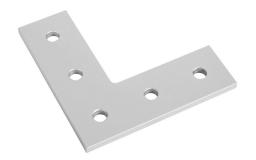
FATH L-shaped flat plate, silver, 5 holes, anodized aluminum, slot size 8. For use with all 1.5in and 3in profile T-slotted rails. Manufacturer part number: 093EVL114114S02.
