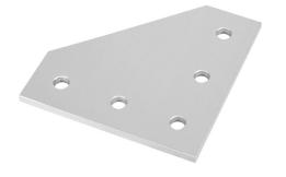
FATH flat plate, silver, 90-degree, 5 holes, anodized aluminum, slot size 8. For use with all 1.5in and 3in profile T-slotted rails. Manufacturer part number: 093EVL114114.
