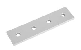
FATH straight flat plate, silver, 4 holes, anodized aluminum, slot size 8. For use with all 1.5in and 3in profile T-slotted rails. Manufacturer part number: 093EVA38152.
