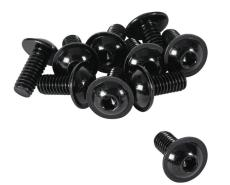
FATH flanged button head socket cap screw, gloss black, 5/16-18 UNC x 11/16in, zinc plated steel, slot size 8/10. Package of 10. For use with all 1.5in, 3in, 30mm, 40mm, 45mm, 60mm, 80mm and 90mm profile T-slotted rails.
