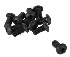
FATH button head socket cap screw, black, 5/16-18 UNC x 5/8in, zinc plated steel, slot size 8/10. Package of 10. For use with all 1.5in, 3in, 30mm, 40mm, 45mm, 60mm, 80mm and 90mm profile T-slotted rails. Manufacturer part number: 4ISO7380U,31-,68M.
