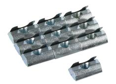
FATH roll-in nut, silver, 1/4-20 UNC, zinc plated steel, slot size 8. Package of 10. For use with all 1.5in and 3in profile T-slotted rails. Manufacturer part number: 09602U1/4F.
