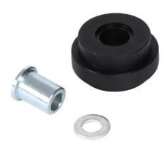
FATH roller, black, 29 x 15mm, glass-filled nylon/steel, slot size 6. For use with all 1in and 2in profile T-slotted rails. Manufacturer part number: 093029.
