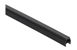
FATH cover and reduction profile, black, 2000mm, polypropylene, slot size 6. Package of 25. For use with all 1in and 2in profile T-slotted rails. Manufacturer part number: 092033.
