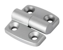
FATH right-hand detachable combination hinge, silver, die-cast aluminum, slot size 6. For use with all 1in and 2in profile T-slotted rails. Manufacturer part number: 095A2525RS20.
