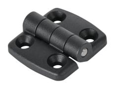
FATH non-detachable combination hinge, black, fiberglass reinforced plastic, slot size 6. For use with all 1in and 2in profile T-slotted rails. Manufacturer part number: 095K2525F06.
