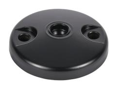
FATH swivel base with anti-slip plate, black, 80mm, die-cast zinc, ball joint size 15. For use with all rails. Requires ball joint size 15 swivel foot threaded rod. Manufacturer part number: 098D080ZBSG.
