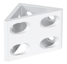
FATH gusseted inside corner bracket, silver, 90-degree, 8 holes, anodized aluminum, slot size 6. For use with all 1in and 2in profile T-slotted rails. Manufacturer part number: 093W8106N06.
