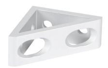
FATH tall gusseted inside corner bracket, silver, 90-degree, 4 holes, anodized aluminum, slot size 6. For use with all 1in and 2in profile T-slotted rails. Manufacturer part number: 093W8103N06.
