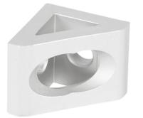
FATH gusseted inside corner bracket, silver, 90-degree, 2 holes, anodized aluminum, slot size 6. For use with all 1in and 2in profile T-slotted rails. Manufacturer part number: 093W8104N06.
