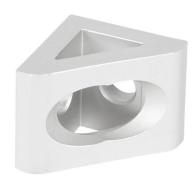
FATH gusseted inside corner bracket, silver, 90-degree, 2 holes, anodized aluminum, slot size 6. Package of 10. For use with all 1in and 2in profile T-slotted rails. Manufacturer part number: 093W8104N06.
