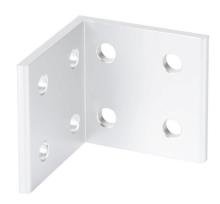
FATH inside corner bracket, silver, 90-degree, 8 holes, anodized aluminum, slot size 6. For use with all 1in and 2in profile T-slotted rails. Manufacturer part number: 093WD5151.
