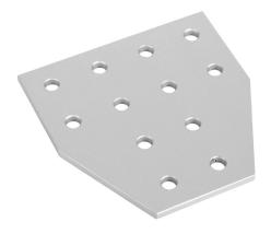
FATH T-shaped flat plate, silver, 12 holes, anodized aluminum, slot size 6. For use with all 1in and 2in profile T-slotted rails. Manufacturer part number: 093EVT102102D.
