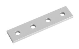
FATH straight flat plate, silver, 4 holes, anodized aluminum, slot size 6. For use with all 1in and 2in profile T-slotted rails. Manufacturer part number: 093EVA25102.
