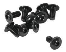
FATH flanged button head socket cap screw, gloss black, 1/4-20 UNC x 1/2in, zinc plated steel, slot size 6/8/10. Package of 10. For use with all T-slotted rails. Manufacturer part number: 4ISO7380U1/4-1/2F.
