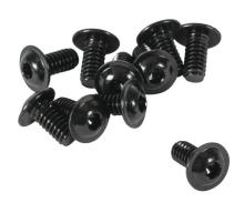
FATH flanged button head socket cap screw, gloss black, 1/4-20 UNC x 1/2in, zinc plated steel, slot size 6/8/10. Package of 10. For use with all T-slotted rails. Manufacturer part number: 4ISO7380U1/4-1/2F.
