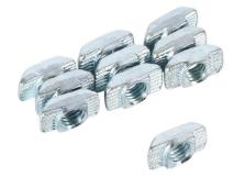
FATH hammer nut, silver, 10-32 UNF, zinc plated steel, slot size 6. Package of 10. For use with all 1in and 2in profile T-slotted rails. Manufacturer part number: 096H0610-3210.
