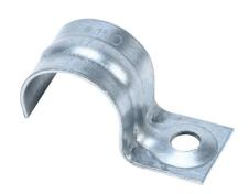
Minerallac 1-hole conduit mount strap, standard duty. Package of 100. For use with 3/4in RMC/IMC/LFMC, 1in tubing, 2/0 AWG SER.
