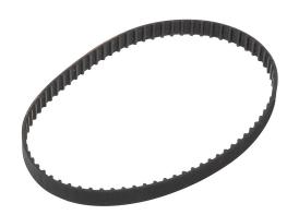
SureMotion timing belt, 1/5in XL pitch, 3/8in wide, 75 tooth, 15in pitch length (circumference), neoprene, fiberglass reinforced.
