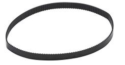
SureMotion timing belt, 0.08in MXL pitch, 1/4in wide, 150 tooth, 12in pitch length (circumference), polyurethane, polyester reinforced. Package of 3.
