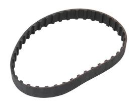
SureMotion timing belt, 3/8in L pitch, 1/2in wide, 40 tooth, 15in pitch length (circumference), neoprene, fiberglass reinforced.
