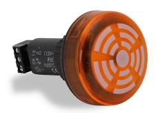
WERMA audible alarm buzzer, 80 dB at 1m, 2.8 kHz tone frequency, continuous tone(s), 115 VAC, permanent LED indicator(s), yellow, 22mm, panel mount, polycarbonate housing, yellow, IP65.
