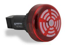
WERMA audible alarm buzzer, 80 dB at 1m, 2.8 kHz tone frequency, continuous tone(s), 115 VAC, permanent LED indicator(s), red, 22mm, panel mount, polycarbonate housing, red, IP65.
