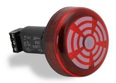
WERMA audible alarm buzzer, 80 dB at 1m, 2.8 kHz tone frequency, continuous tone(s), 24 VDC, permanent LED indicator(s), red, 22mm, panel mount, polycarbonate housing, red, IP65.
