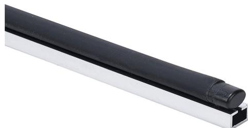
ASO Safety Solutions safety contact edge, 15 x 10mm, 4ft length, pigtail, 8.2ft/2.5m cable length. Aluminum mounting rail included. Preassembled with 8.2k ohm resistor for 2-wire installation.
