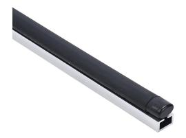
ASO Safety Solutions safety contact edge, 15 x 10mm, 3ft length, pigtail, 8.2ft/2.5m cable length. Aluminum mounting rail included. Preassembled with 8.2k ohm resistor for 2-wire installation.
