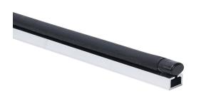
ASO Safety Solutions safety contact edge, 15 x 10mm, 2.5ft length, pigtail, 8.2ft/2.5m cable length. Aluminum mounting rail included. Preassembled with 8.2k ohm resistor for 2-wire installation.
